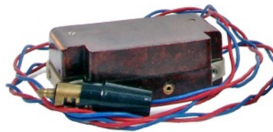
General view of 31215 receiver with battery cassette (in front of receiver) and a 12V vehicle battery adapter (below).
